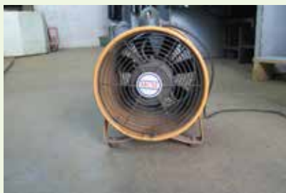
抽氣扇 Ventilation fan/ Industrial mobile air conditioner (寶路華 Blower)
