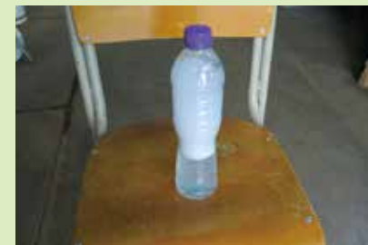
試漏梘水 Soap water for gas leakage check
